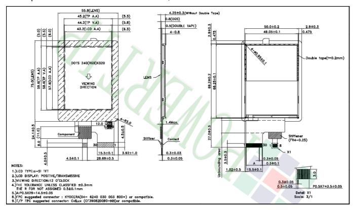
• 4.3" TFT with OGS – Part no. PH480272T-006-IAC02 Cost effective solution for 4.3" capacitive touch panel LCD module.
